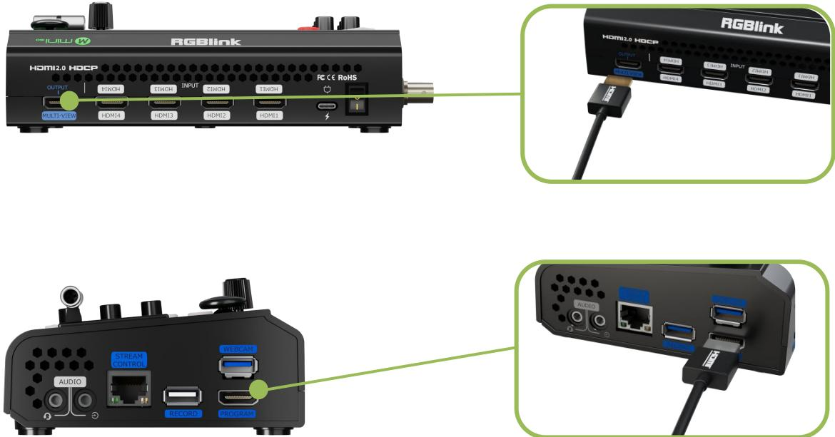
The default output of MULTI-VIEW is a multi-view monitoring display, so that the user can see the audio and video of all input sources as well as the current status of the mini-ISO's various functions, as well as the preset views and the current main output screen.
