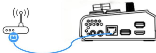
2. Go to Settings > IP Settings to access the following interface. Enable DHCP to automatically obtain an IP address. The mini-ISO can only connect to Ethernet and bind to TAO Cloud once the interface displays an IP address assigned by the router.
